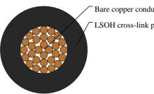
Bare copper conductor LSOH cross-link polyolefin insulation
